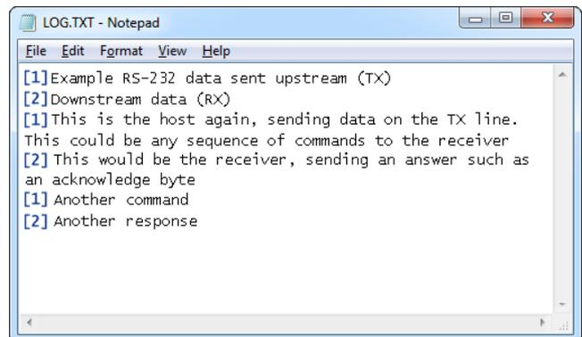
The upstream data (TX) and downstream data (RX) will be differentiated by the channel headers interleaved in the log file.
