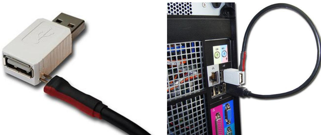
Take the supplied USB cable and connect it to the mini-port on the keyloggers side. **Make sure the red mark on the cable faces the keyloggers USB port.** Then, connect the USB cable to a free USB port. Finally, connect the keylogger to a second USB port. **Do not connect the keyboard.** After a few seconds, the hardware keylogger will automatically get detected as a mass storage device, and pop up as a removable drive.
