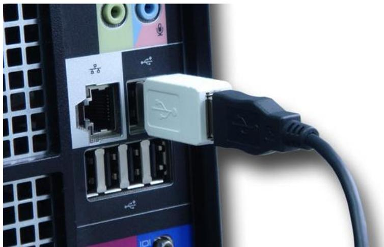
Plug the USB keylogger in-between the keyboard and USB port. Do **not** use the supplied USB cable (it is for configuration purposes only).
