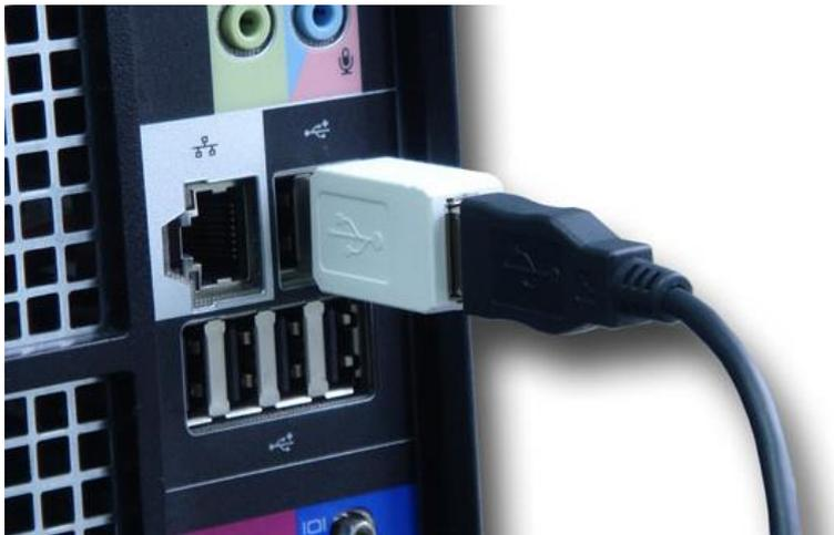
Plug the USB keylogger in-between the keyboard and USB port. Do **not** use the supplied USB cable.
