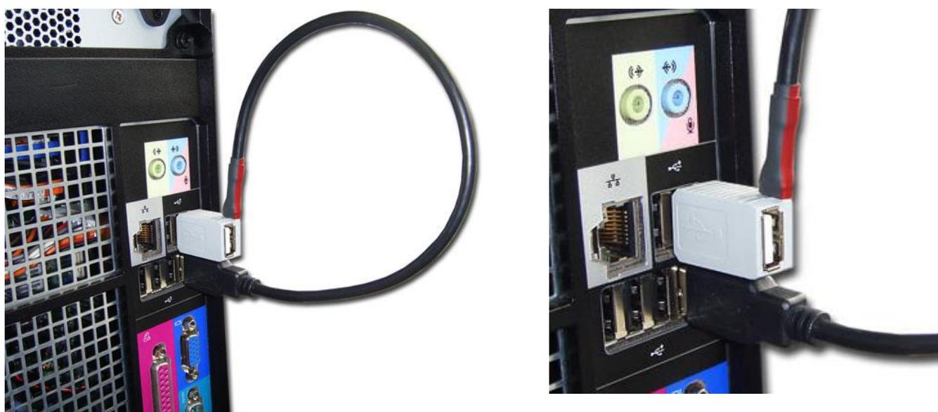
Then, connect the USB cable to a free USB port on the computer.
