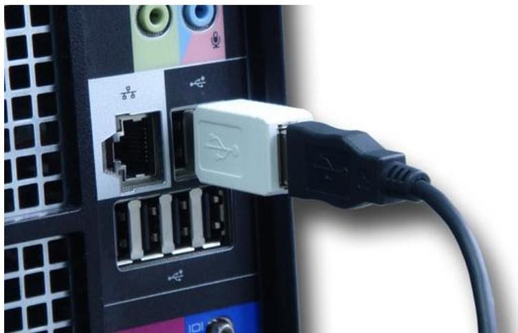
Plug the keylogger in-between the keyboard and USB port, and press the 3-key combination **simultaneously** (by default K, B, S). After a few seconds, the hardware keylogger will automatically get detected as a mass storage device, and pop up as a removable drive.
