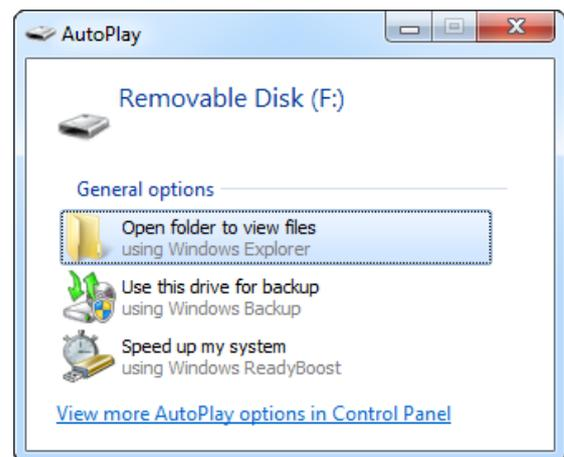
Depending on the drive letters available, the device will be visible as a new drive, for example F:. Use the systems file manager to browse this disk (for example *Explorer*). The keyboard will be disconnected and unavailable, so the mouse must be used to browse the disk.
