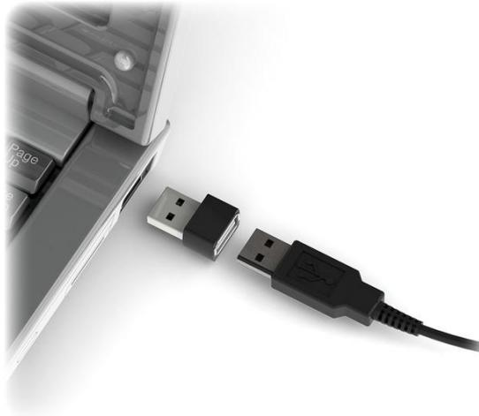
**To view recorded data**, plug the device in-between the keyboard and USB port, and press the 3-key combination **simultaneously** (by default K, B, S)
